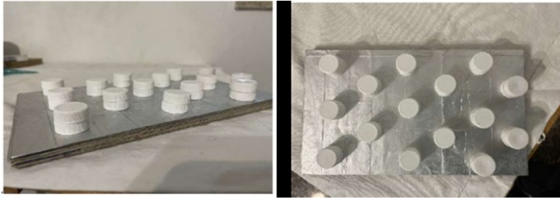
Fig. 4. Images of the basic unit of the prototype of the insulating panel for underfloor heating made using a poly laminate panel and the caps of discarded containers
