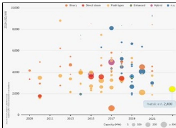
Fig. 1. Total installation costs by project, technology, and geothermal energy capacity
